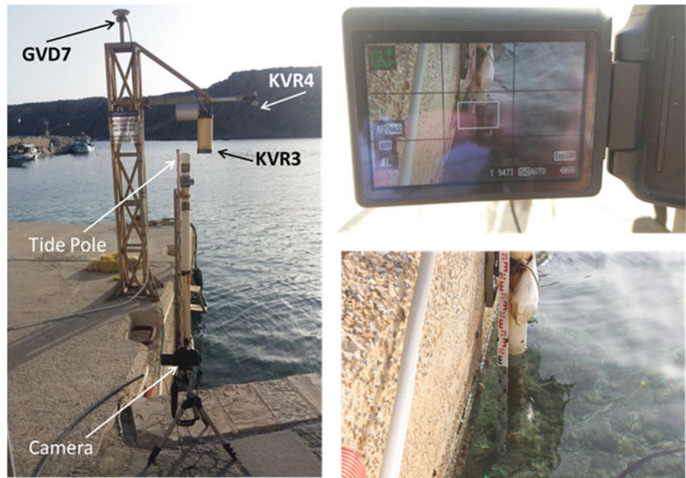
Fig. 2 Field calibration of tide gauges in Gavdos Cal/Val, Greece. A digital camera placed in front of a tide pole to capture actual sea surface level can be used to calibrate the operating tide gauges
