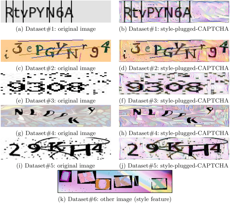
Fig. 2. The sampling example of style-plugged-CAPTCHA for the original image of each dataset when selecting dataset #6 as the style image.
