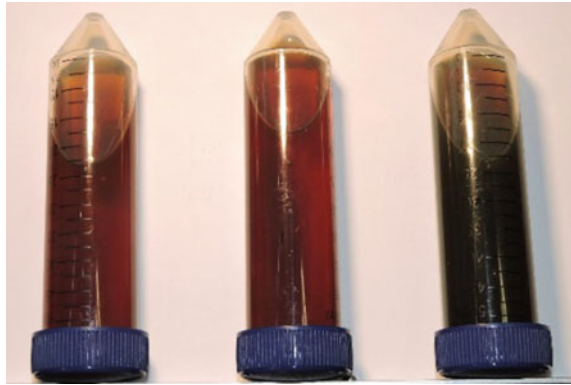
Fig. 3 Aspect of the fluid used in the tests: Left: new fluid from the package; Centre: fluid after the 230 h test at OTR; Right: Fluid sampled from the tractor reservoir after 900 h in real work conditions
