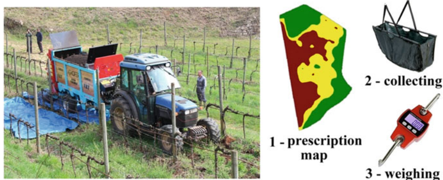
Fig. 5 The amount of matrix distributed by the machine in each inter-row surveyed, and collected on the plastic sheets of known surface (left), was later weighed by using a digital dynamometer and compared with the expected figure resulting from the prescription map (right)
