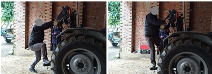
Fig. 3 One participant raising the FROPS, using the rear three-point lower links as a support for the feet
