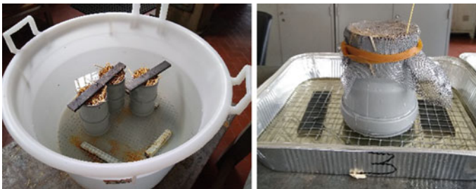
Fig. 4 Water holding capacity and porosity measurements apparatus
