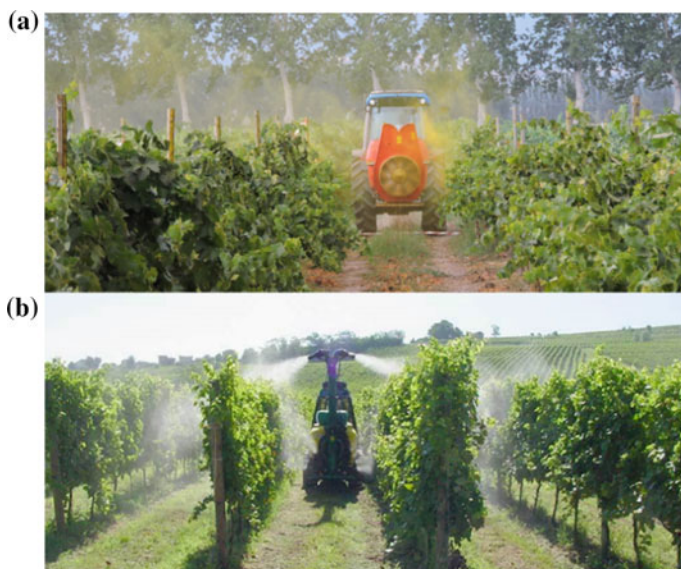
Fig. 2 Conventional mounted airblast sprayer Dragone k2 500 (a) and multiple-row pneumatic sprayer Cima 50 Plus 400 L equipped with spray head TC.2M2C (b) during field pesticide application
