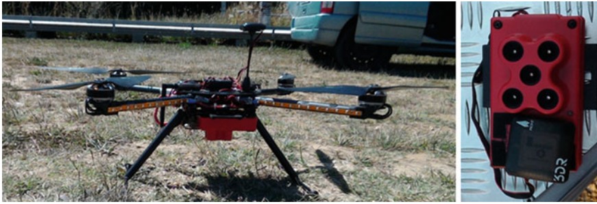
Fig. 2 On the left the UAV equipped with the multi-camera, on the right, in detail, the Micasense-RedEdge used during the survey
