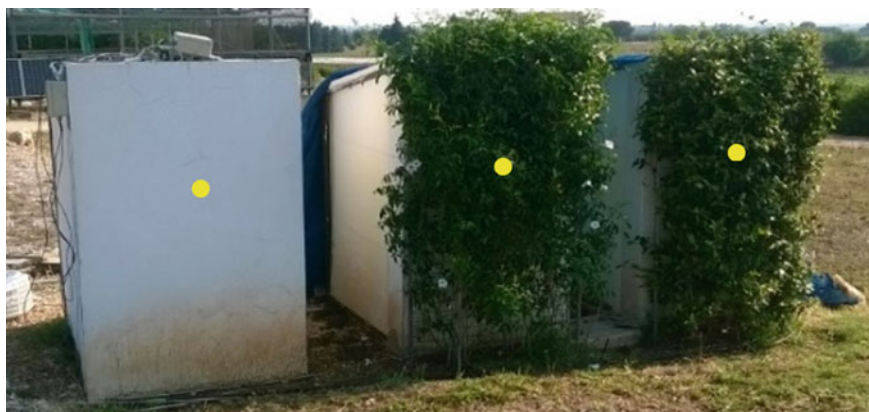
Fig. 1 The experimental walls at University of Bari and the location of the sensors measuring the temperature of the external plaster surfaces (yellow point); the left wall is the control wall, the central green façade is screened with Pandorea jasminoides variegated and the right façade with Rhynchospermum jasmynoides
