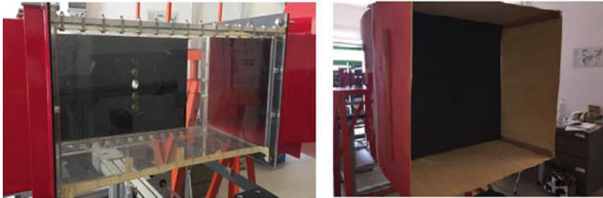
Fig. 1 Picture of the wind tunnel test chamber and the honeycomb at the beginning of the tunnel
