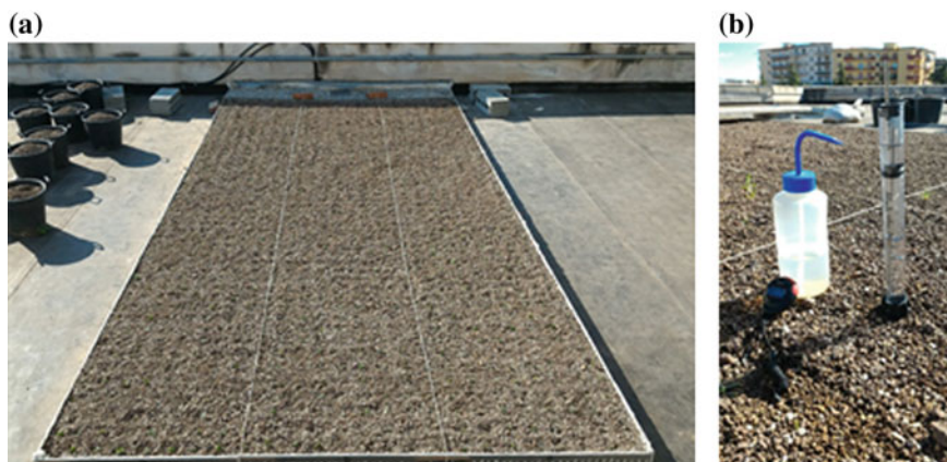
Fig. 1 Experimental green roof plot at the time the first sampling campaign (Age 0) (a); MDI device used for infiltration tests (b)
