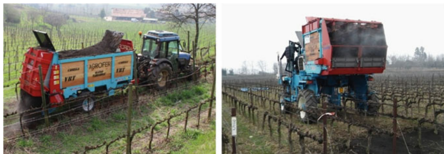
Fig. 2 Two of the spreader prototypes manufactured for the Vitisom project: the towed self-levelling (left) and the straddle self-propelled (right) models
