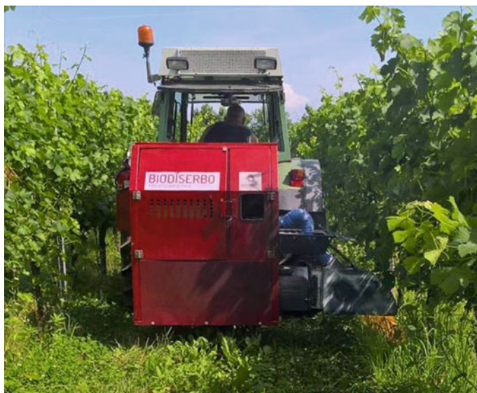
Fig. 1 The biomass flamer in the vineyard
