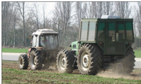
Fig. 1 An example of the layout of a drawbar power test on field by dynamometer application
