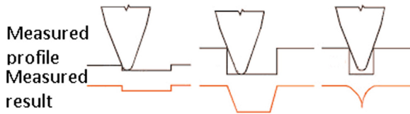
Fig. 4. Distortion of information about geometry in the measurement of a complex part.
