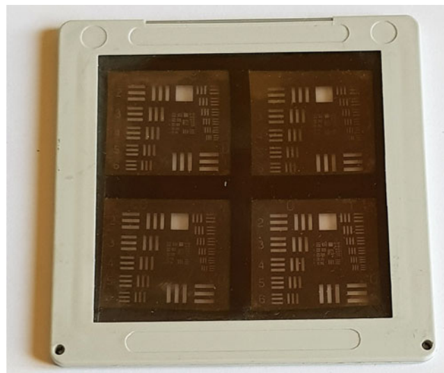
Fig. 7.3 Resolution target for testing optical performance (USAF 1951 test target). The edges of the bigger elements can be used as an edge step to calculate overall response of the system and then the LSF
