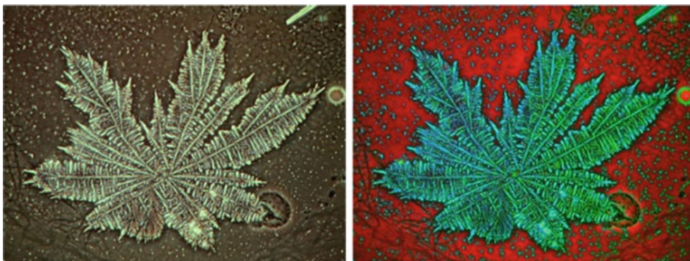
Fig. 6.21 Thin layer crystallization, objective 40/0.65, phase contrast, HFW: 0.25 \text{ mm} , standard view (left), multicolor sandwich (right) based digital superimposition of three single images taken with monochromatic red, green, and blue light
