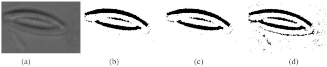
Fig. 8.1 Diatom binarization by gray level thresholding: (a) original image, (b) Otsu, (c) maximum entropy, and (d) Phansalkar
