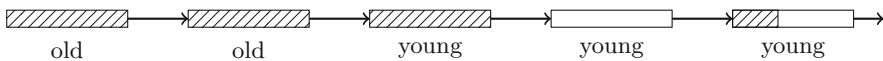
Fig. 4. From-space contains black region pages from old generations, black region pages from young generations, white region pages from young generations, and partly-white region pages from young generations. No white region pages from old generations exist.
