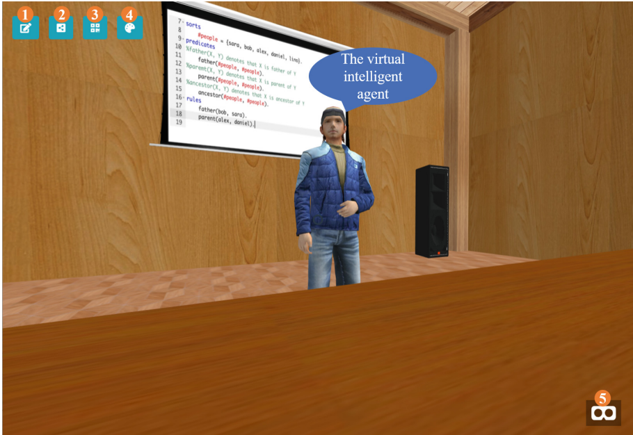
Fig. 1. The VRASP learning interface. (1) ASP editor, (2) sharing with a URL, (3) sharing with a QR code, (4) VR editor, and (5) changing between VR and 3D mode
