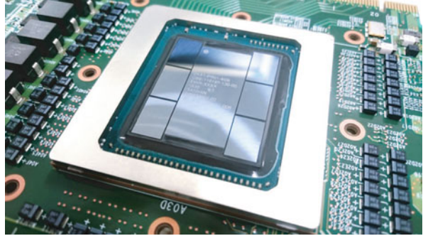
Fig. 1 A vector processor in a VE (provided by NEC)
