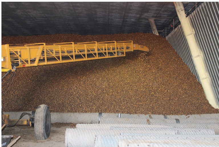
Fig. 17.9 Potatoes are bulked pile into a storage using a tier system and minimizing rollback and bruising
