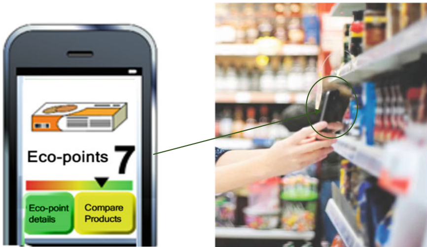
Fig. 6.14 Consumer acquire the product’s eco-points via scanning the RFID tag embedded in the product with smartphone, which helps consumer to seek sustainable products
