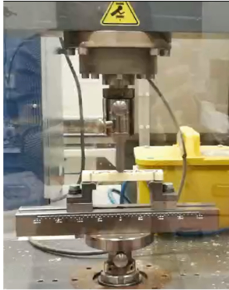
Fig. 2. Three-point bending test setup
