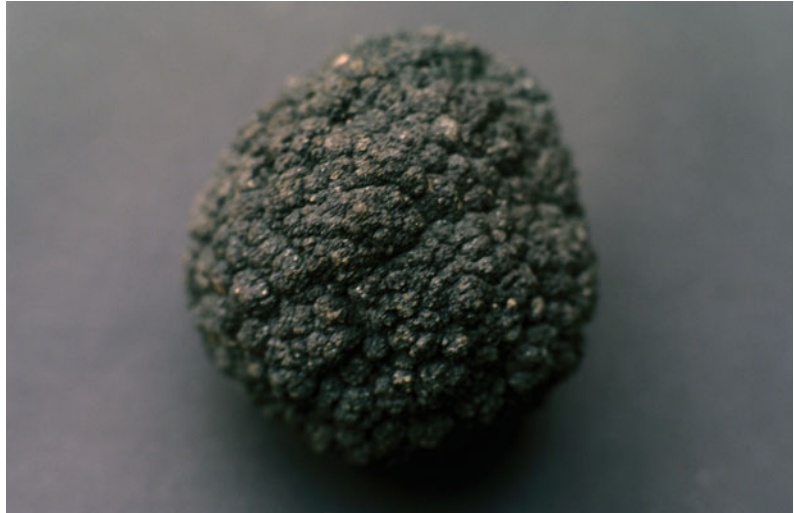
Fig. 14.10 Polymetallic manganese nodule from the Pacific Ocean . Nodules grow incrementally at rates of 1-10 mm per million years. Image width approximately 20 cm. Credit Koelle (CC BY-SA 3.0, https://creativecommons.org/licenses/by-sa/3.0 )
