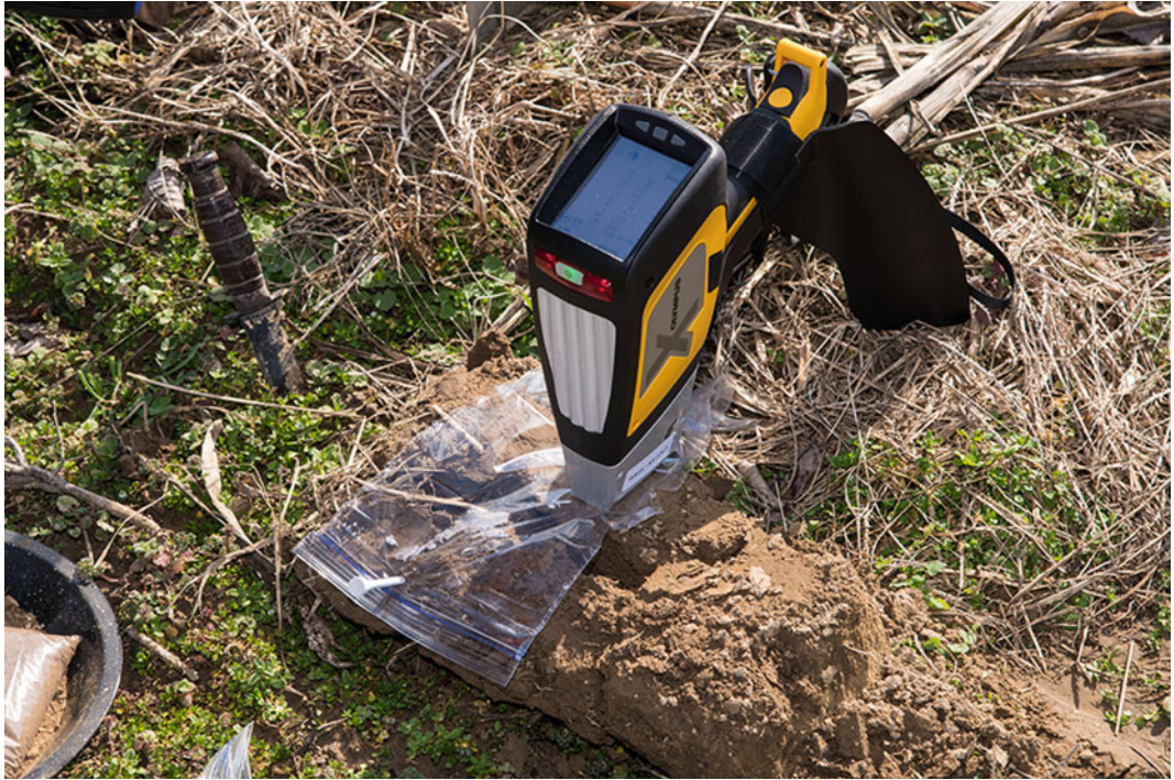
Fig. 8.2 Handheld XRF device. In this example the handheld XRF is used to evaluate the amount of metal
