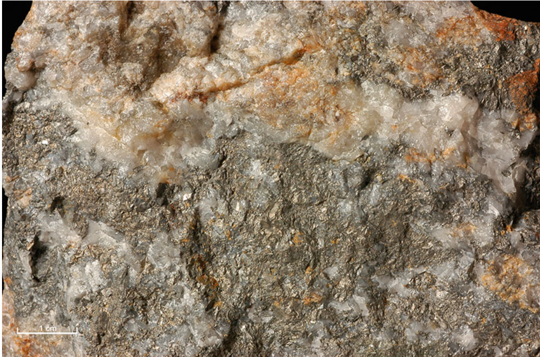
Fig. 3.4 Arsenopyrite, an iron arsenic sulphide, is identified as the metallic mineral in this specimen from Talnoy, UK. Quartz veining and granodiorite fragments are also visible. © NERC (used with permission)
