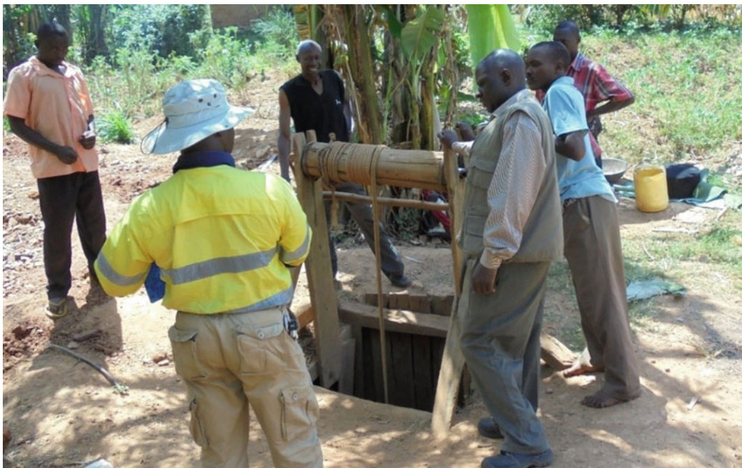
Fig. 12.8 Manual winching of ore from an ASGM gold mine. Credit: Martin Nyakinye (DGS)
