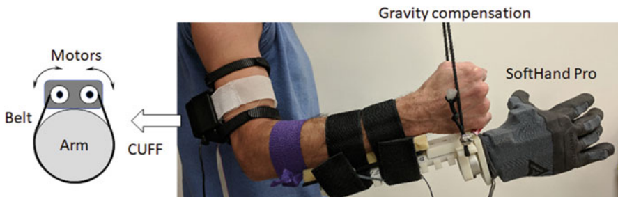
Fig. 1 Components of the implemented closed-loop prosthetic system. (Adapted from [13])
