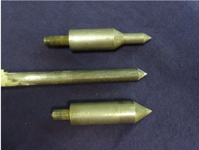
Fig. 6.2 Heads of measuring bars used in the inverse experiments
