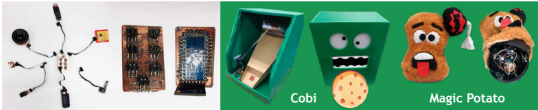
Fig. 4. IoT4Fun Toolkit adapted by the Cobi and Magic Potato teams.
