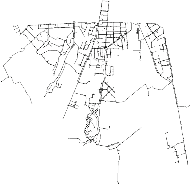
Fig. 1. EPANET model of the Pressure Management Zone (PMZ) “Abbiategrasso”, in Milan, Italy
