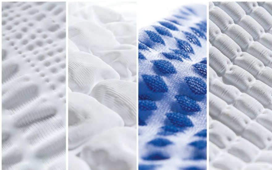
Fig. 8 Laser-molded PET and polyamide textiles [51]
