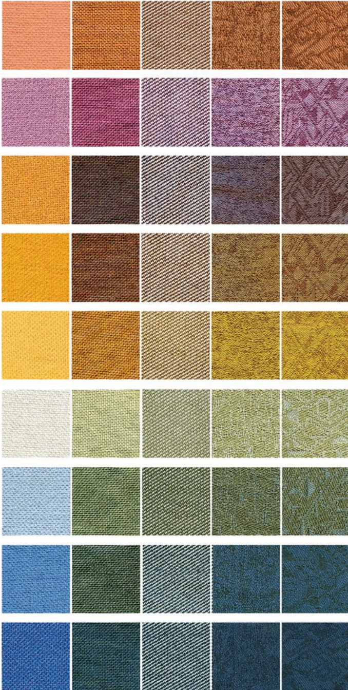
Fig. 12 Examples of one-step laccase-catalyzed coloration on nylon, wool, wool/polyester, and specially constructed woven jacquard designs, using different dye bath conditions. (Source: Prajapati, C)
