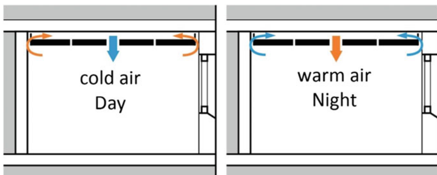
Fig. 4.18 PCM-incorporated ceiling or roofs
