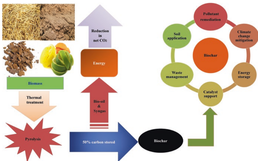
Fig. 4.1 Schematic diagram showing general route of biochar preparation and its potential application
