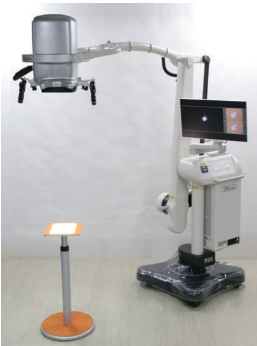
Fig. 25.2 The medical imaging projection system (MIPS). Photograph of the MIPS, showing the projection head and pole components. The MIPS has a projection head that uses a half mirror to match the optical axis of the near-infrared fluorescence imaging camera and the projector. The MIPS obtains the location of the fluorescence indocyanine green emission and projects its image onto the location of the fluorescence emission in real time, regardless of shifting and deformation of the organ. The projector of the MIPS can also illuminate the surgical field, allowing surgeons to perform the procedure without the need for operating lights
