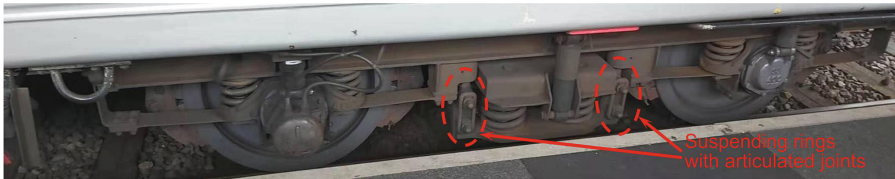
Fig. 13. Passenger frame bogie with lateral swung bolster in Sweden rails
