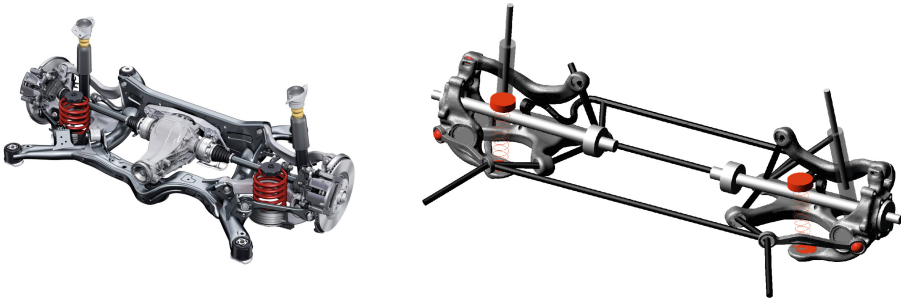
Fig. 3. Audi self-tracking trapezoidal-link rear suspension: Real system (left) [32], Multibody simulation model in Adams/View (right)
