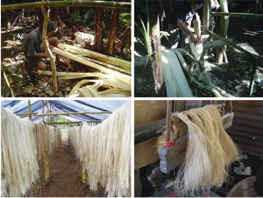
Fig. 2 Harvesting of the abaca plant and separation into sheaths (Wikimedia Commons 2018c), manual separation of fibers (Wikimedia Commons 2018d), drying (Wikimedia Commons 2018e), and abaca fiber (Wikimedia Commons 2019), respectively
