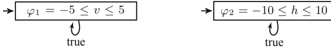
Fig. 2. Two scenario objects, represented as transition systems (state machines) that, respectively, put hard limits on the vertical and horizontal angular velocities of the drone. Each scenario has a single synchronization point, as indicated by its single state, in which it contributes a constraint (e.g., \varphi_1 = -5 \leq v \leq 5 ) to the global constraint set. The only transition, a self loop that does not depend on the variable assignment returned by the solver, indicates that the scenario continues to contribute this constraint, regardless of the satisfying assignment discovered by the solver.
