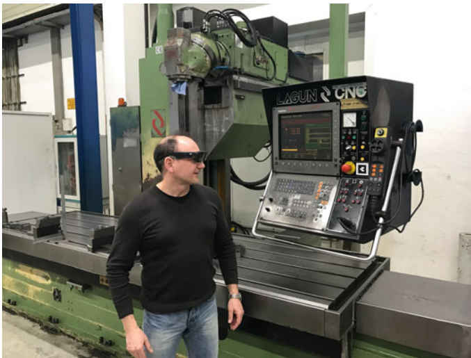
Fig. 6 Demonstration of the maintenance application on a typical manufacturing machine using smart glasses
