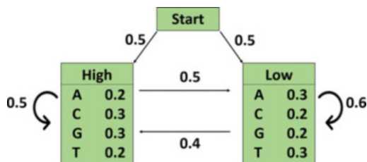
Fig. 1 Schematic representation of High and Low states, showing transition probabilities between states and probabilities of getting each nucleotide while in each state (after Borodovsky and Ekisheva [8])
