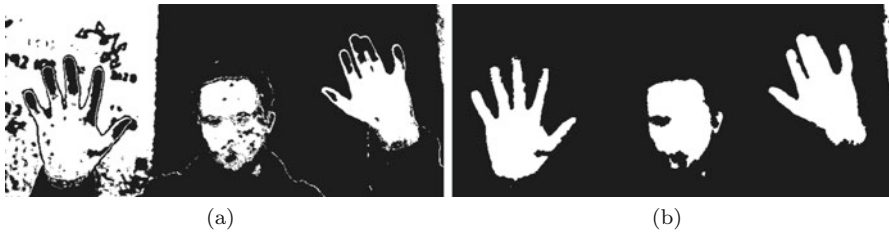
Fig. 5 Comparison between the original adaptive histogram-based skin detection and the proposed enhanced skin detection: (a) adaptive histogram-based skin detection result; (b) result obtained from the enhanced skin detection procedure
