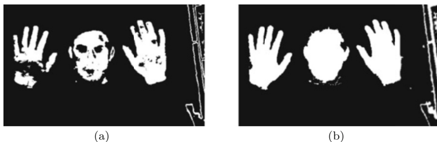
Fig. 11 Comparison between the proposed enhanced skin detection and adaptive histogram-based skin detection: (a) skin image of the original adaptive histogram-based skin detection; (b) skin image of the enhanced skin detection method
