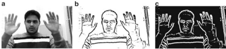
Fig. 1 Adaptive Gaussian thresholding and image inversion: (a) the grayscale image of the input; (b) the corresponding thresholded image with strong intensity changes darkened using adaptive Gaussian thresholding; (c) the inverted image in which strong intensity changes, i.e., edges, are highlighted
