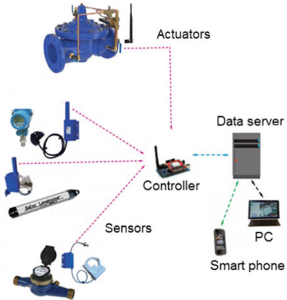
Fig. 12.4 Architecture of a smart network (IoT)
