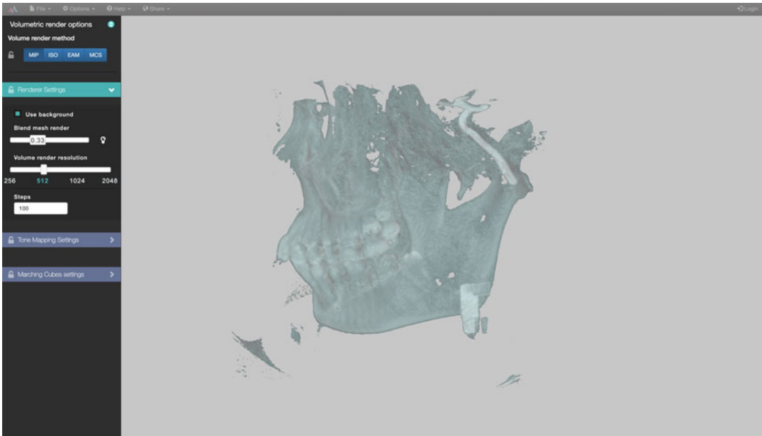
Fig. 1.16 A rendering composed of mesh geometry rendered using Med3D integrated renderer overlaid by maximum intensity projection rendered using VPT
