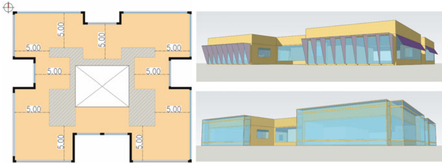
Fig. 45.1 Left office typical floor plan layout with the requirement set in SI 5282 Energy Rating of Buildings for 5 m depth of windows to usable floor space. Right top: shading devices on south and west elevations. Right bottom: view of typical floor plan's façades with DSFs on all orientations
