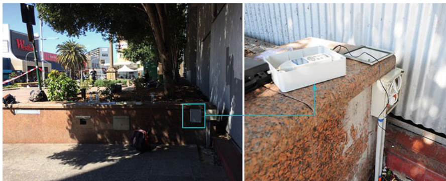
Fig. 11.3 Sound level meter installed in the Plaza, Memorial Square. (Authors 2018)
