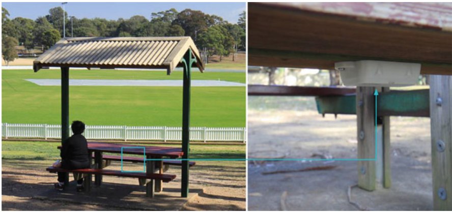
Fig. 11.2 Vibration sensor installed under the seats, Olds Park. (Authors 2018)
