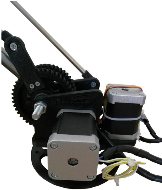
Fig. 5. Ready-made base with fixed stepping motors
