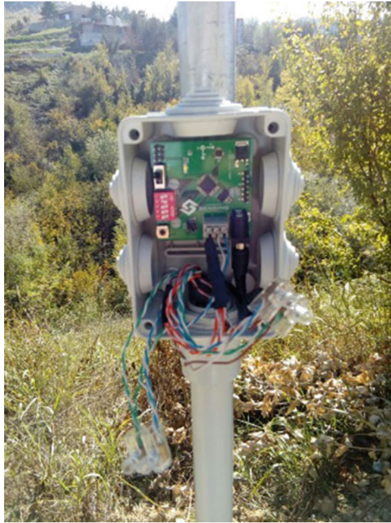
Fig. 3 The proposed sensor node installed in a real environmental Ftp web server data output example
