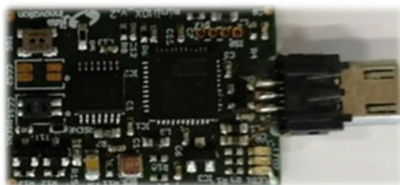
Fig. 1 The commercial electronic nose JLM Minimox from JLM innovation used in this study
