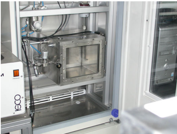
Fig. 1 Photo of the 15 lt “Large Volume Test Chamber” (LVTC)
