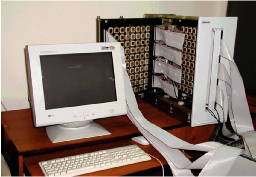
Fig. 3.4 FOP based upon RPA MiniTera-2 and computer workstation
