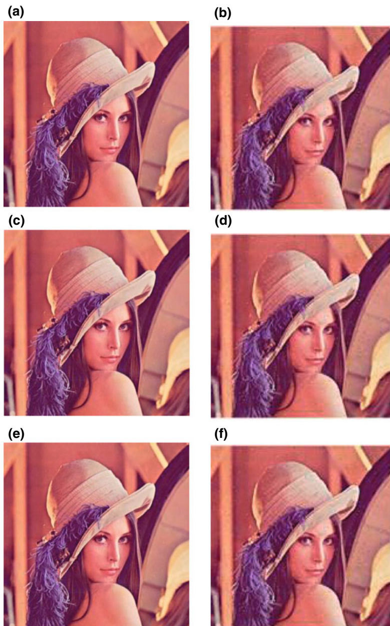
Fig. 5.1 Original and noisy images. Noise: Salt-Pepper. a Original image; b noisy images, PSNR = 25.36; c noisy images, PSNR = 18.34; d noisy images, PSNR = 15.41; e noisy images, PSNR = 12.64; f noisy images, PSNR = 9.22
