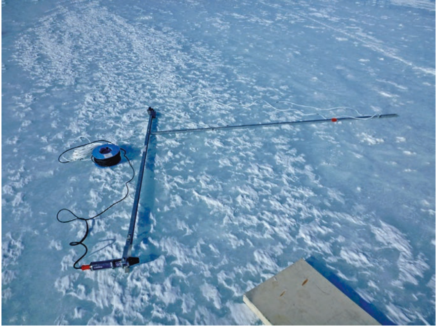
Fig. 6.12 L-arm mounted with a TriOS spectroradiometer for measuring spectral resolved irradiance below the ice. Distance between hole in the ice and point of measurement is 1.5 m. The L-arm is operated through a drilled hole and the arm unfolds below the ice and obtains a configuration as shown in the photo. (Photograph by: Authors)
