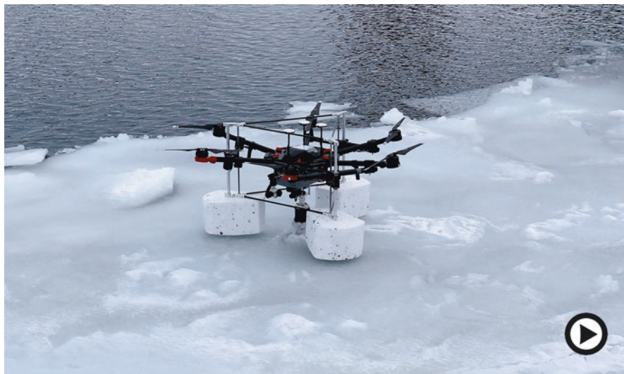
Fig. 6.3 A video showing the work and sampling on the thin ice using ice drone (Photograph by: Dan Carlson). Video: Stratoz Visuals – M.Skovby ( https://doi.org/10.1007/000-05k )
