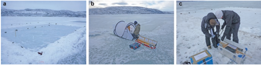
Fig. 4.19 Experimental site with transparent tarpaulin and shaded ice (Intermediate light) (a), work on the sea ice with the Imaging-PAM fluorometer in a tent (b), and cutting a sea ice core on the ice (c) Note the black cloth to protect the ice core from sunlight. (Photographs by: Authors)
