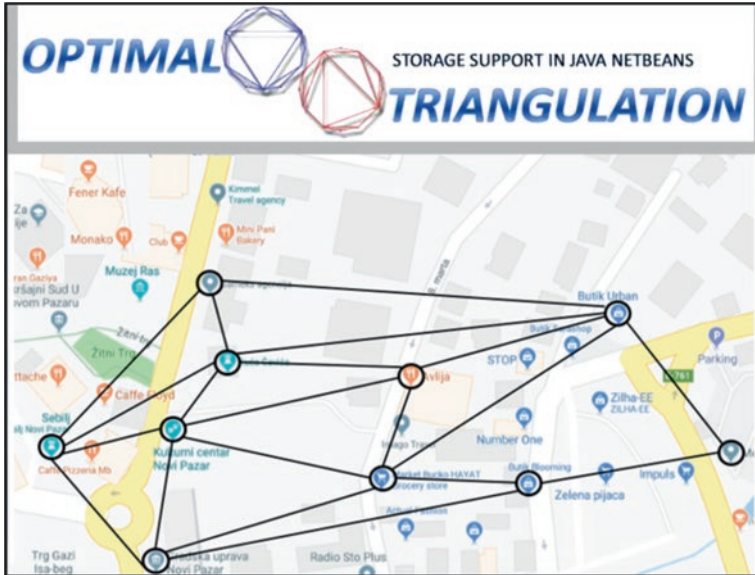
Fig. 17.12. Java application for finding optimal triangulations
