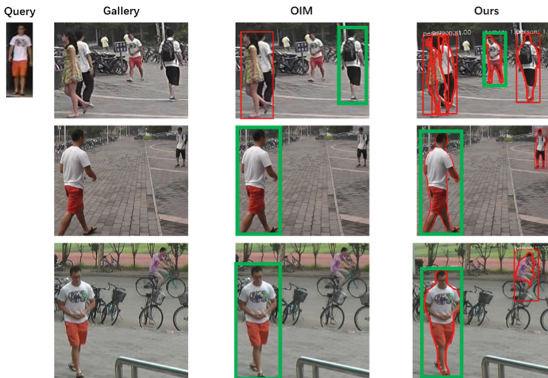
Fig. 5. Comparison of person search results between our method and OIM. The red rectangles are the results of person detection, and the green rectangles are the results of person search. For all these three gallery images, it is clear that some person identities have not been detected by OIM. And for the first gallery image, the person search result for OIM is also wrong. (Color figure online)
