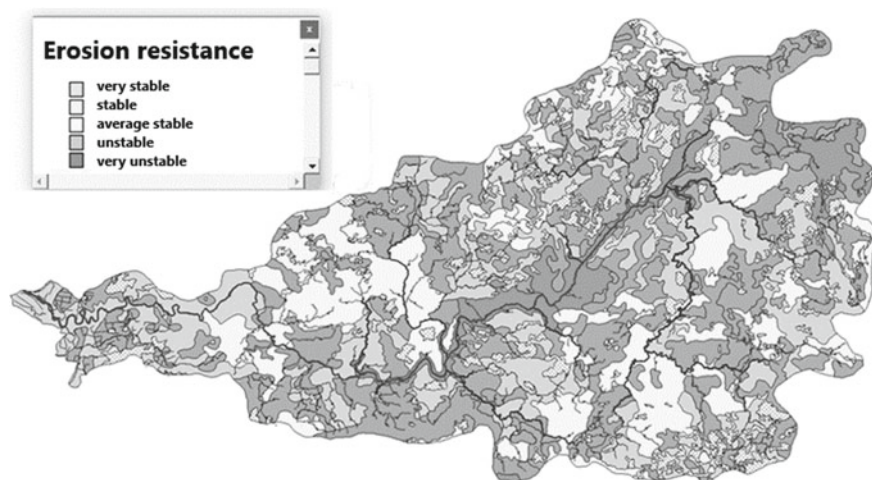
Fig. 7.5 Synthetic map of land resistance of landscapes of the study area to water erosion
