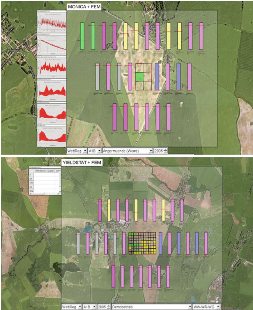
Fig. 24.11 Visualisation of simulation results for the combined FEM-MONICA model (top) and the combined FEM-YIELDSTAT model (bottom) at local level for a small part of farms within the Uckermark region, Germany (regionalisation method: WETTREG, climate scenario: A1B; green bars: ecological parameters, pink bars: economic parameters, yellow bars: crop yields, grey bars: fertilisation/nutrition parameters, blue bars: water-related parameters)
