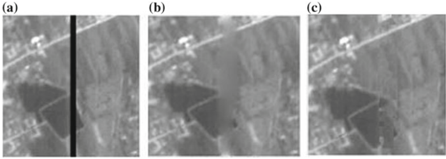
Fig. 1 Comparison of removing dead line from CBERS (China Brazil Earth Resource Satellite) image a 8-pixel dead line image b inpainting using PDE c inpainting using exemplar based technique
