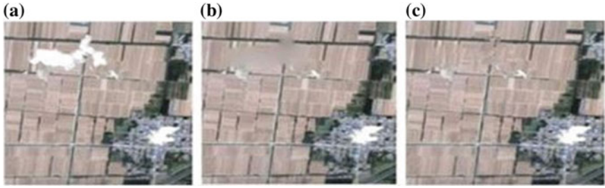
Fig. 5 Using GaoFen-2 RS imagery, comparison of clouds removal a Original image. b inpainting using SiLRTC [20] c inpainting using MRF [19]
