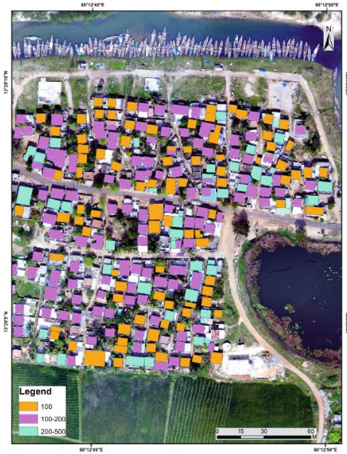
Fig. 4 Electricity Consumption of each household in units; Orange(up to 100), Pink (100–200) and Green (200–500)
