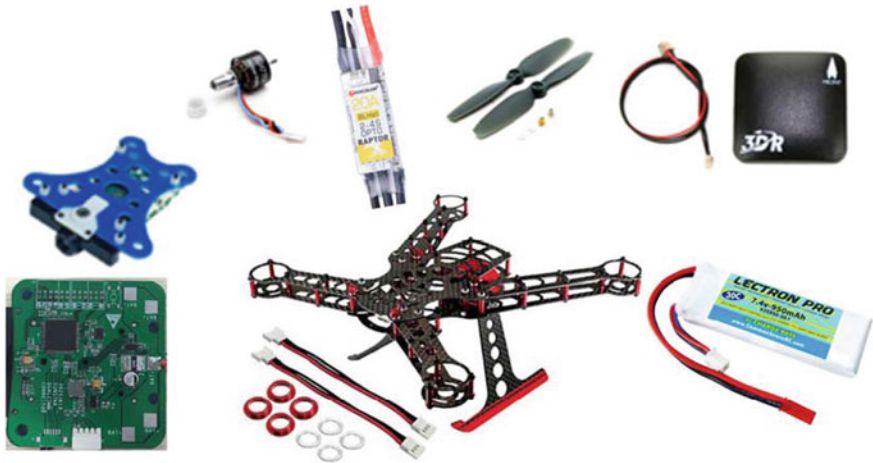
Fig. 4 Parts of UAV
