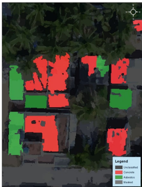
Fig. 6 Automatic extraction of concrete roof top
