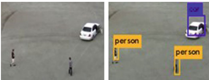
Fig. 7 Sample image frame snapshot from UAV in left and detected/identified object at right
