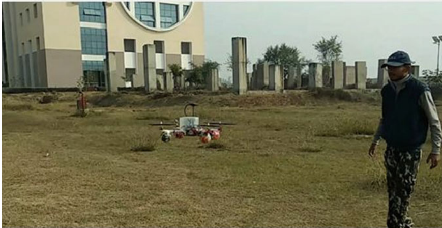
Fig. 9 Testing of UAV: navigation of quadcopter to prospective fire location
