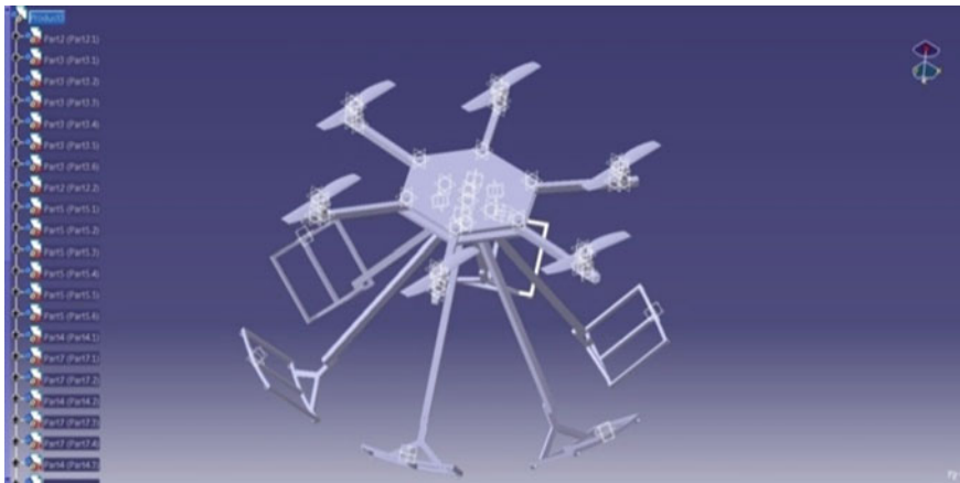
Fig. 5 Combined view of hexacopter with retract landing gear
