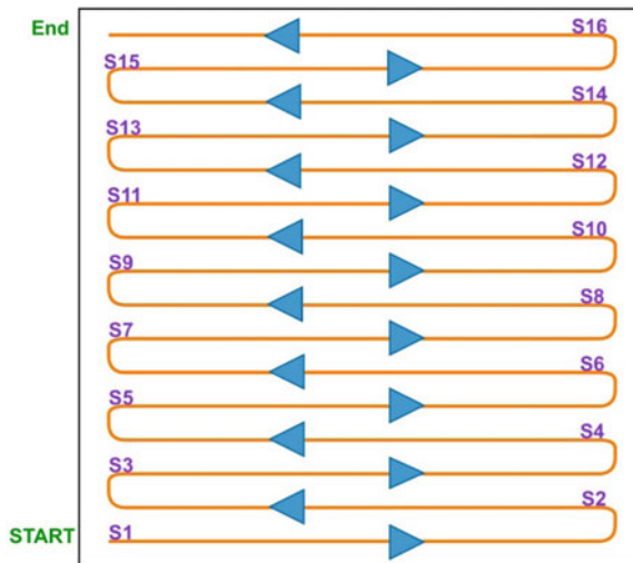
Fig. 4 Proposed scanning map for mother drone (the field is divided into several lanes, S1, S2, S3, etc.)
