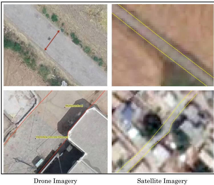
Fig. 4 Demarcation of buildings and roads through drone and WV-II satellite data
