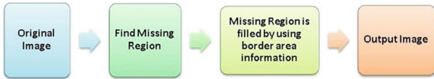
Fig. 3 Block diagram of diffusion-PDE based image inpainting technique
