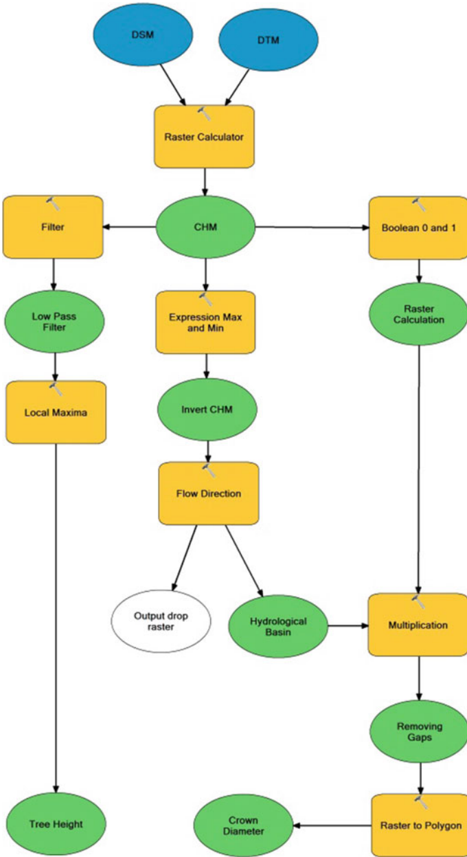
Fig. 4 Model for extraction of tree height and crown diameter
