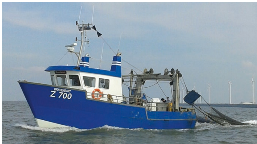
Fig. 18.1 Small Belgian otter trawler ( \leq 221 kW, < 70 GT, < 48 h) targeting brown shrimp and flatfish in the North Sea. (Photo credit: F. Willemkens)
