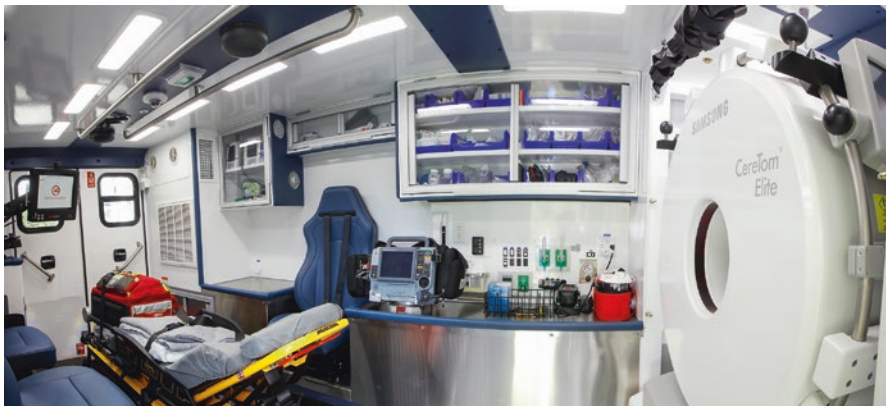
Fig. 30.1 Interior of the University of Rochester MSU showing the portable CT scanner (to the right)
