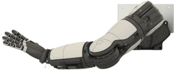
Fig. 44.4 Rendering of the artificial arm. The black parts represent the structural shell made of hard plastic while the white parts represent the soft artificial skin
