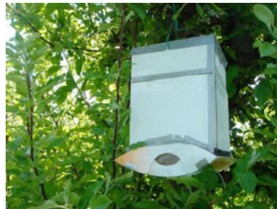
(b) Prototype of the IoT neural network Codling Moth smart trap.
