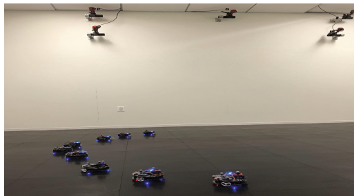
Fig. 4. Experimental environment with small robots and motion capture system
