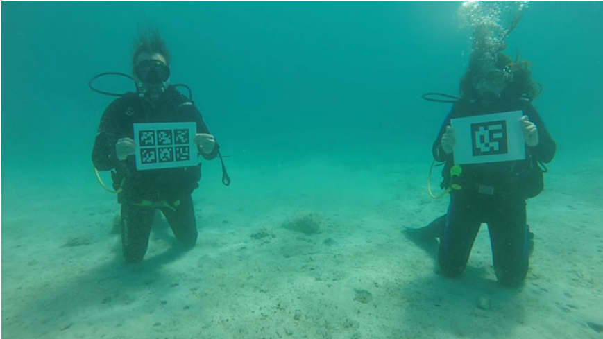
Fig. 11.1 Two divers holding sheets with markers for initial assessment of image-improving algorithms
