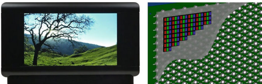
Fig. 3.5 Brightside DR 37P HDR display (left) and the LED array behind the LCD panel (right). Image courtesy of Brightside
