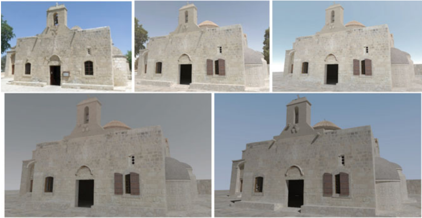
Fig. 2.6 Top left: photograph. Top middle: Image-based Lighting (captured from site). Top right: Preetham Sky Model (Preetham et al. 1999). Bottom left: CIE clear sky model. Bottom right: Directional light source mimicking the sun
