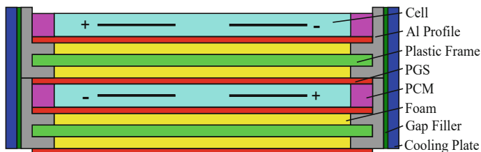
Fig. 1 Concept of the module in cross-section view
