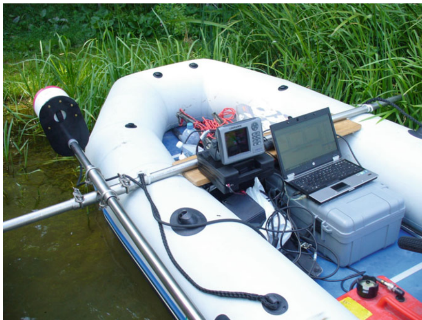
Fig. 4 ADCP RiverPro by Teledyne mounted on a surveying boat ready for measurements at Charzykowskie Lake on 2015 08 28
