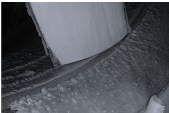
Fig. 7 Fan blade and casing with \text{ZnSO}_4 crystals adhesion
