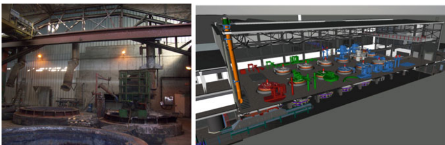
Fig. 3 Left: Old lead refining facility; Right: New lead refining capacity with expansion setup where 12 kettles could be utilized
