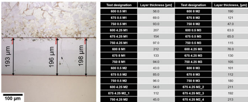
Fig. 4 Extract for the thickness measurement of the resulting intermetallic layer (left) and average thickness of the resulting Co–Zn alloy layer (right) analysed and measured by LOM [19]
