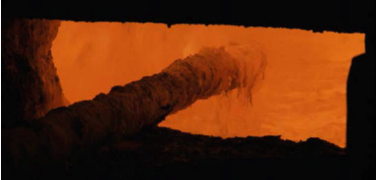
Fig. 1 Ionic liquid as being injected into a copper bath (for demonstration purposes)
