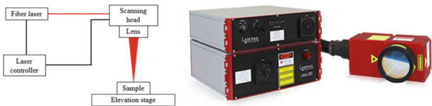
Fig. 1 Schematic of the experimental setup used (left) and photograph of the LXQ-20W laser marking system (right)
