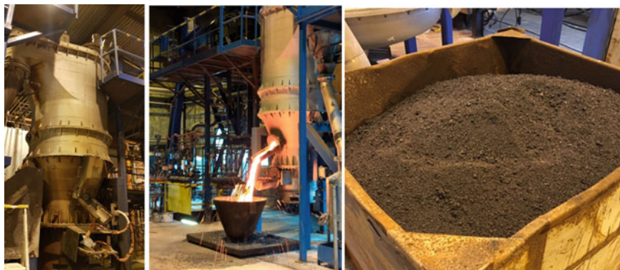
Fig. 8 Pilot ScanArc furnace at Hofors, Sweden. In the middle tapping of jarosite slag and on the right water granulated slag after fuming. The slag volume is around 1/7 of the feed volume and around 1/2 of the weight of the feed
