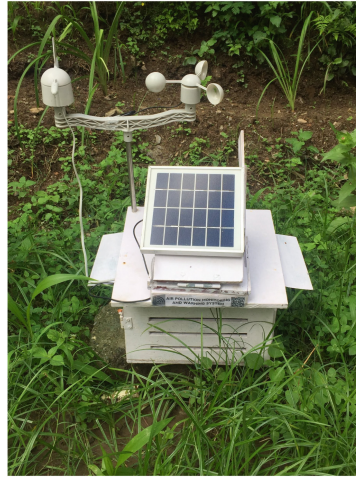
(b) The actual AQMPWS constructed based upon its hardware design.
