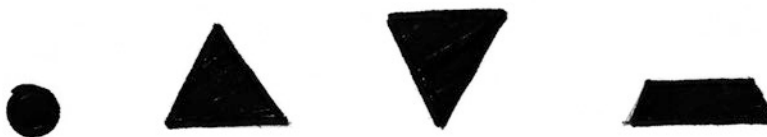
Fig. 2 Cut section of the needle tips. From left to right; taper (round), cutting, reverse cutting, spatulated
