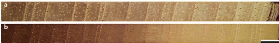
Fig. 3.5 Cedrela odorata samples showing different colors between heartwood and sapwood and between trees. (a) Marginal parenchyma with more contrast than in (b). Scale 5.0 mm
